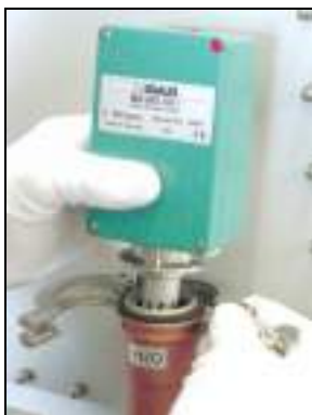
Insert measuring probe and re-clamp.
