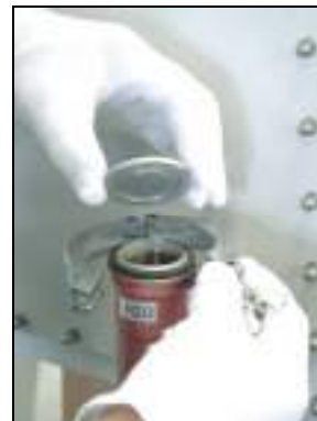
Remove clamp and dummy plug.
