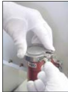
Tighten flange clamp.
